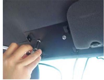
Attaching the control head mounting plate between the sun visors.
