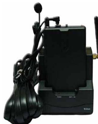
Figure 8 : 900MHz Spread Spectrum Transmitter & Receiver / Charging Base
