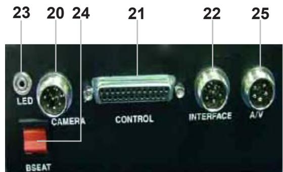
Figure 12 : Rear Panel of Control Head
