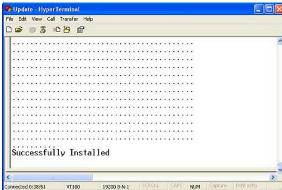
**NOTE:** If for some reason you are disconnected from the Prosecutor downloading, power is lost to the Prosecutor or PC or the firmware update does not finish for any reason you can repeat the procedure above again. The bootstrap loader never is erased and will always request for a valid firmware update until achieved. To do this just power up the Prosecutor while the terminal program is connected and you will see the prompt messages as above window.
