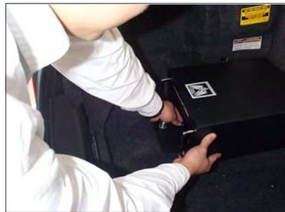
Put the vault on mounting plate and lock them together by using the mounting plate thumb-screw.
