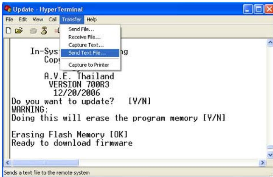
wait Installing until message "Successfully Installed" appear.
