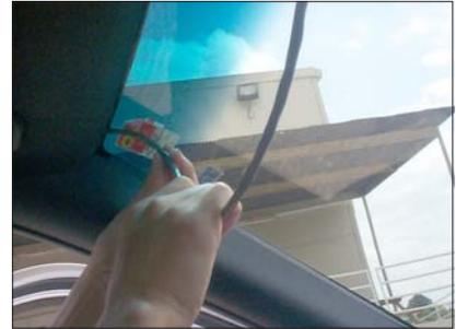
View of DB-25 cable, under headliner, heading toward control head.
