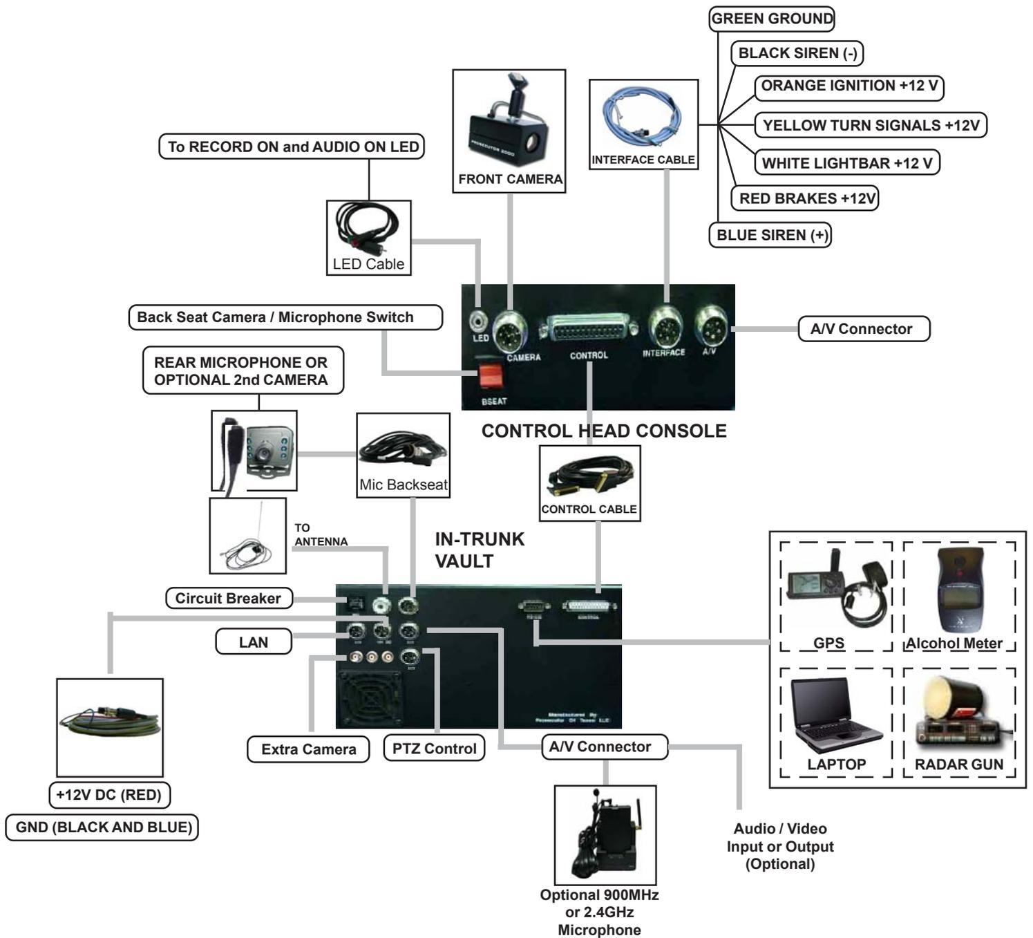
Figure 15 : Description of Connections
