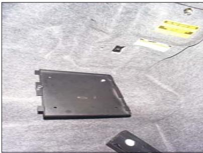
Put the carpet back on, punch holes through carpet to match drilled holes. Place (2) 1/2" x 1" hex head bolts on the left 2 holes of mounting plate, (remember thumbscrew of the mounting plate should face to the bumper direction) and match holes drilled in trunk floor. Place flat washer, then lock washers and hex nuts (or lock nuts) on bolts from outside of trunk floor. Tighten bolts to secure mounting plate.
